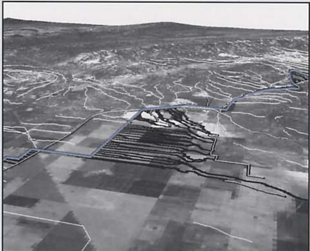
Example of pipeline leaks every 500 feet. (blue = pipeline, black = oil, white = streams)
