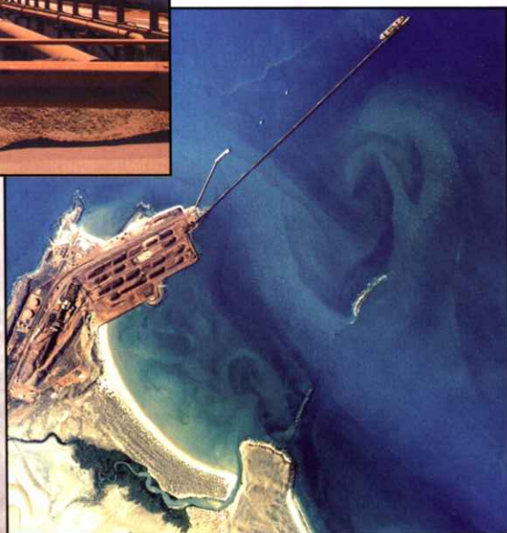
The Ore Wharf at Port Walcott stands 20m above sea level to avoid inundation during cyclonic events. Visiting vessels are laden with diesel fuel and heavy fuel oils.
